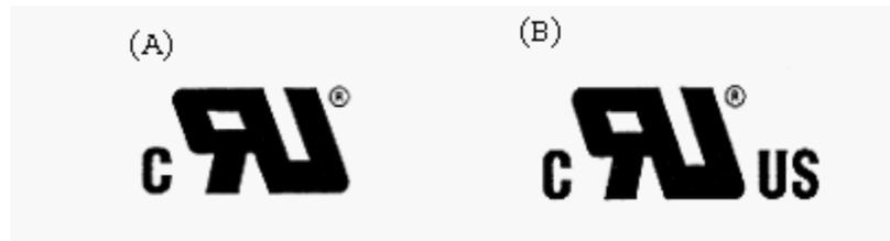
Minimum size of the Recognized Component Mark is not specified as long as it is legible. Minimum height of the registered symbol ® shall be 3/64 inch but may be omitted if it is out of proportion to the Recognized Component Mark or not legible to the naked eye.
