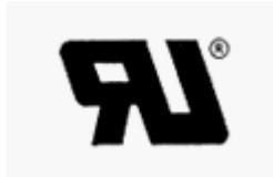
Minimum size of the Recognized Component Mark is not specified as long as it is legible. Minimum height of the registered symbol ® shall be 3/64 inch but may be omitted if it is out of proportion to the Recognized Component Mark or not legible to the naked eye.
